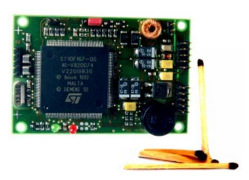
Multitag capable reader module for Smart Labels of 13,56 MHz transponder technology with
